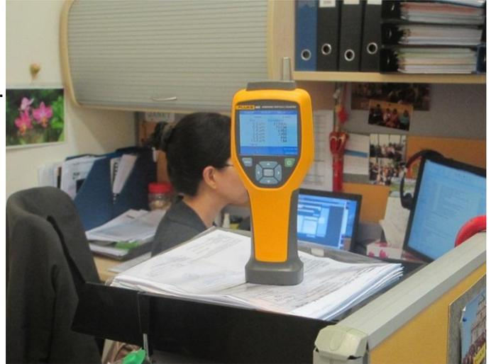
To properly identify and troubleshoot IAQ problems, the technician needs a tool that not only reads particle concentrations for spot check, but also provides continuous monitoring for process control.
