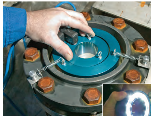
Double the brilliance by simply placing a 4" Phaeton XTL inside a 6" Phaeton XTL.
