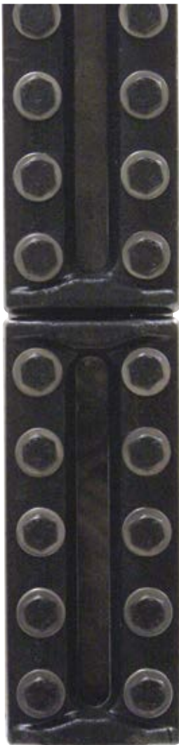
A Typical Dirty Glass Level Gage Without Illumination
