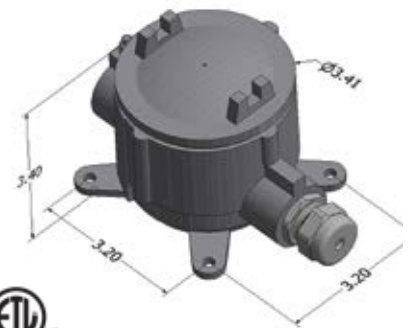
S24928: Terminal Enclosure; 316SS for model EPL-316
