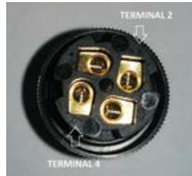
Pin detail for Field Wireable Connector
